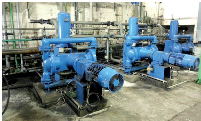
Fig. 3: High volume pulsation dampeners provide a low pulsation performance of the pumps
